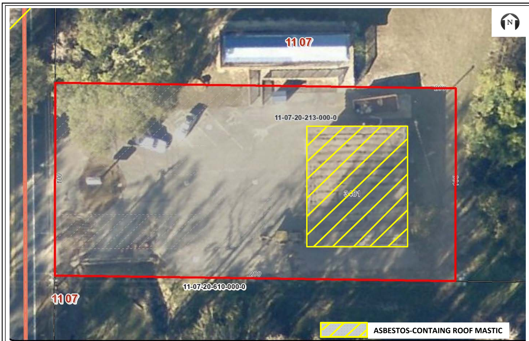
FIGURE 1. ASBESTOS CONTAINING MATERIAL LOCATION MAP 3401 N. MERIDIAN ROAD, TALLAHASSEE, LEON COUNTY, FLORIDA
